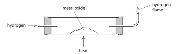
The mass of the metal oxide is measured before and after heating it in hydrogen.
